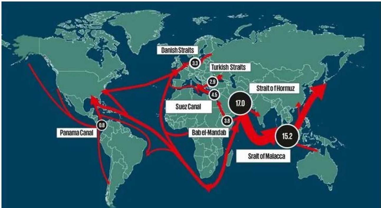
Figure 2: Transport routes and bottlenecks for fossil oil shipping. The numbers indicate the estimated oil volumes in million barrels per day (1 million barrels equals 1,628 GWh 5 ).
